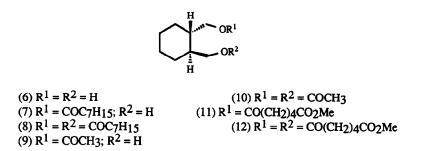
Immobilised *Mucor miehei* lipase (Lipozyme) proved to be the most effective catalyst. Thus esterification of the diol  $(\pm)$ -(6) with octanoic acid in hexane using Lipozyme<sup>®</sup> as the catalyst gave a smooth conversion into the monoester of low optical purity and a slower conversion of the mono-ester into the (S),(S)-diester of good optical purity (*ca.* 83% e.e.).<sup>6</sup>
